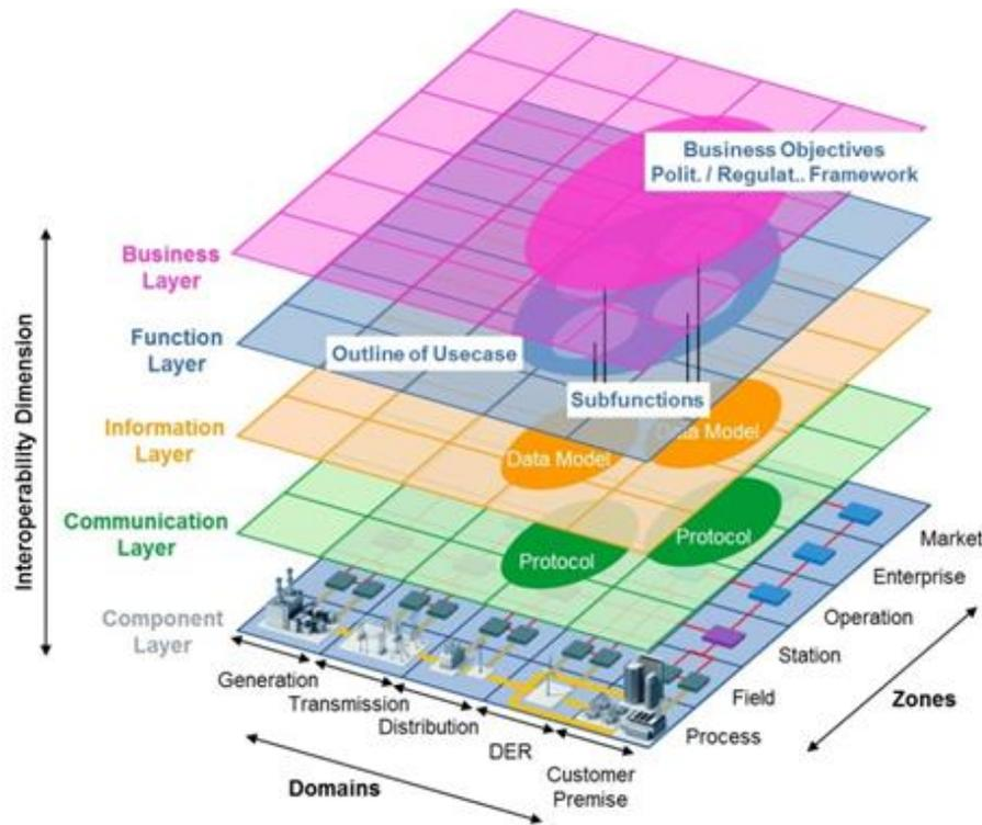
Figure 2-2: Smart Grid Architecture Model (SGAM) [2]
