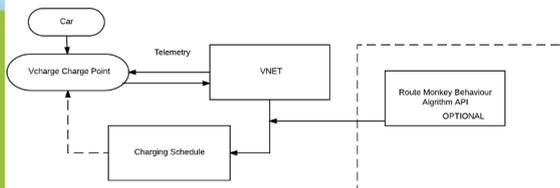
Figure 24: EV system architecture, scenario 2
