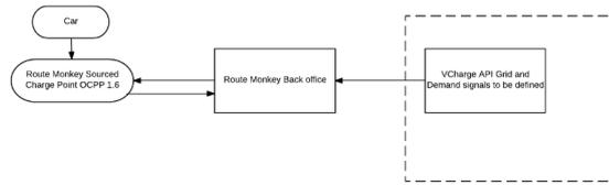
Figure 23: EV system architecture, scenario 1
