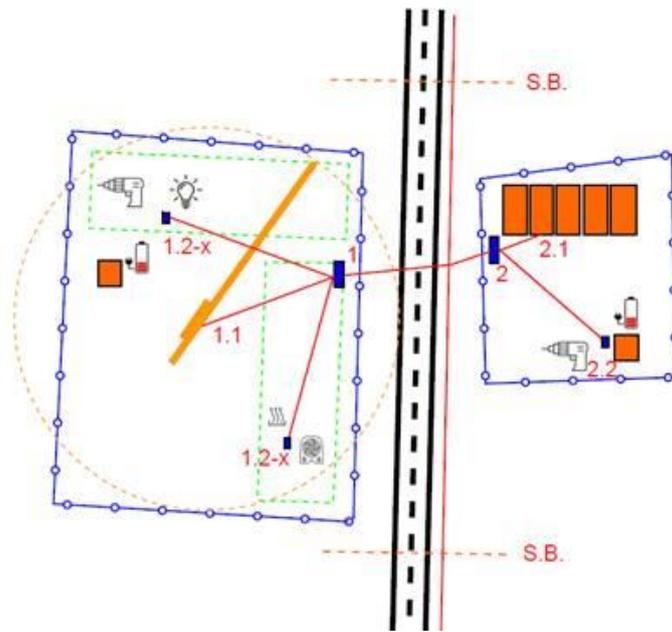
Figure 4: Sub-metering program includes high granularity metering of 1.1, 1.2, 2.1 and 2.2
