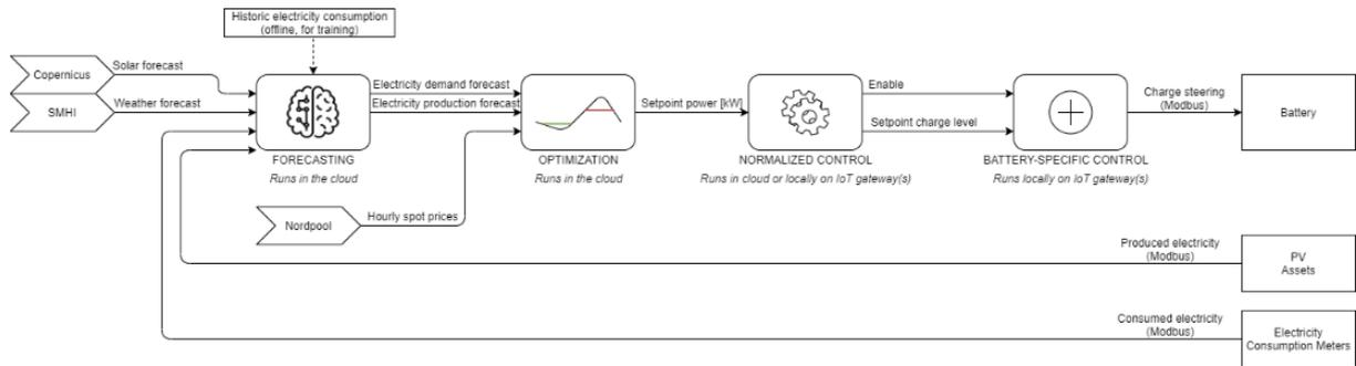
Figure 6: Architecture of local balancing to be developed, evaluated and demonstrated in the project
