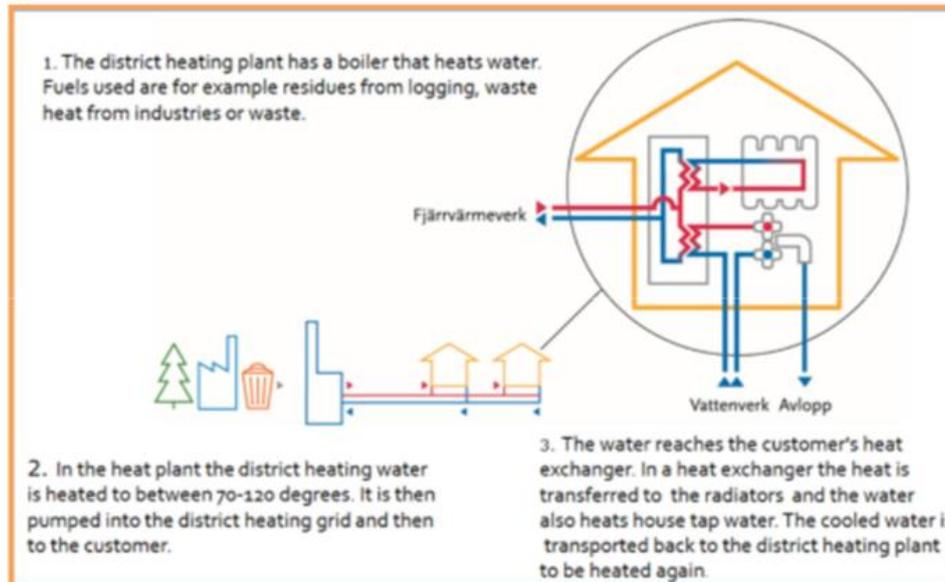
Figure 10: Illustration of the district heating network in Jokkmokk
