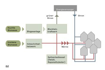
Figure 7: Heat and power distribution concept in the Jündhe energy system (source: Eigner-Thiel, et.al)
