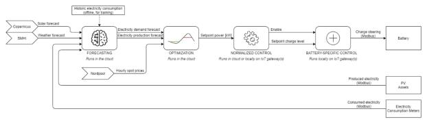
Figure 6: Architecture of local balancing to be developed, evaluated and demonstrated in the project
